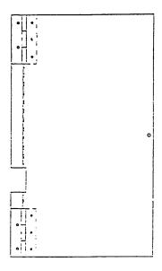
Validator Door and Hinge Assembly 492,051,20x.x3
